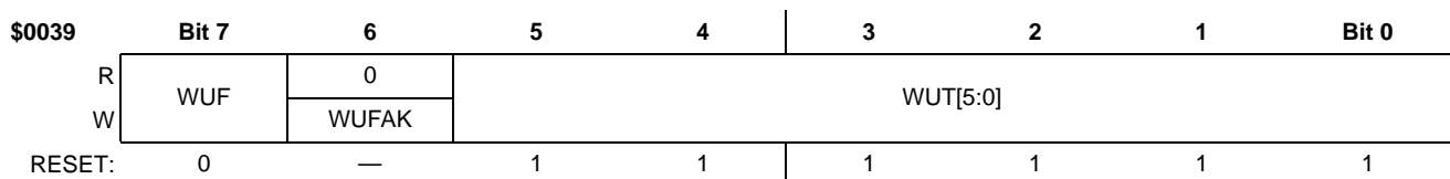
Figure 62. PWU Control/Status Register 0 (PWUCS0)
